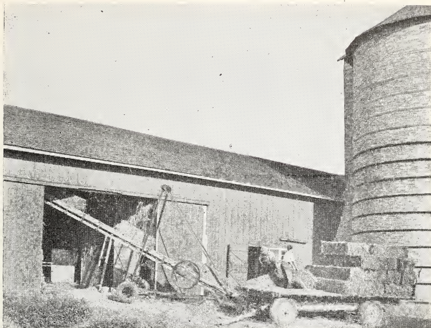
FIGURE 20.—A bale elevator such as this will elevate up to 6 tons of hay per hour, depending on the speed of operation. Two men will be required in the mow to take care of the hay elevated at the rate of 2.5 to 3 tons per hour.
